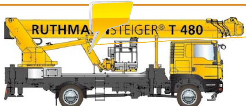
Unmatched flexibility in use by means of extended **RÜSSEL®** (jib)
