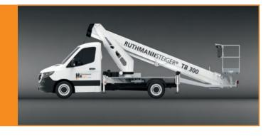
First machine of 30 meters in the 3.5 t range. Also at maximum basket load!
