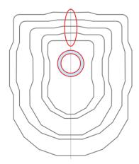
Internal central telescopic cylinder = better extension and retraction = mounted in a protective way
