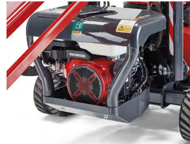
Reinforced protection for the heat engine.
