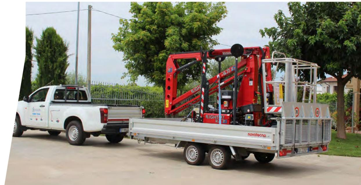
Weighing in at just **1.380 kg**, it can be transported with a category B vehicle or on a dolly trailer.
