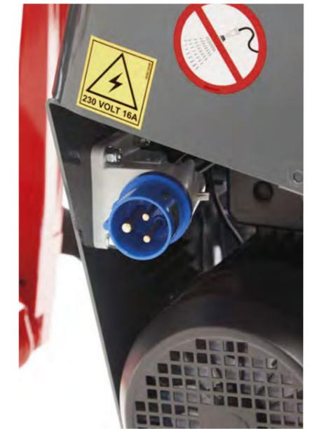
Socket for electric motor and to recharge any lithium battery packs.
