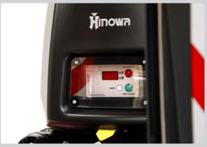
Battery charger and display indicating the charge
