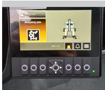
Outrigger setup from inside the cabin
