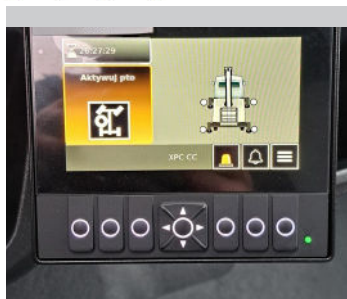
Outrigger setup from inside the cabin
